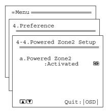
**Activated:** Select when speakers are connected to the ZONE2 SPEAKERS terminals. During playback in the remote zone (Zone 2), the listening mode for the main zone becomes either Stereo or Direct.
